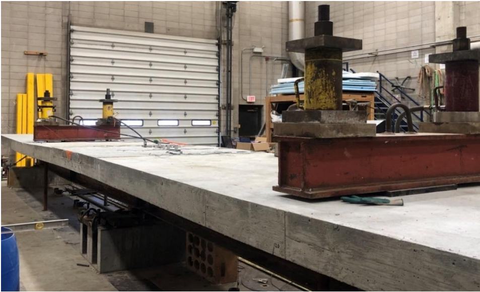
Figure 2.15 Laboratory Test Setup Showing Actuators on Loading Points
