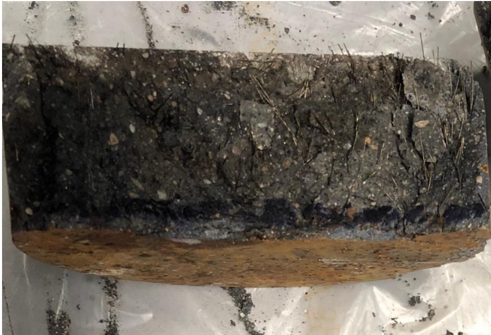
Figure 4.4 Chloride migration in a sample of NP1 in rapid chloride migration test
