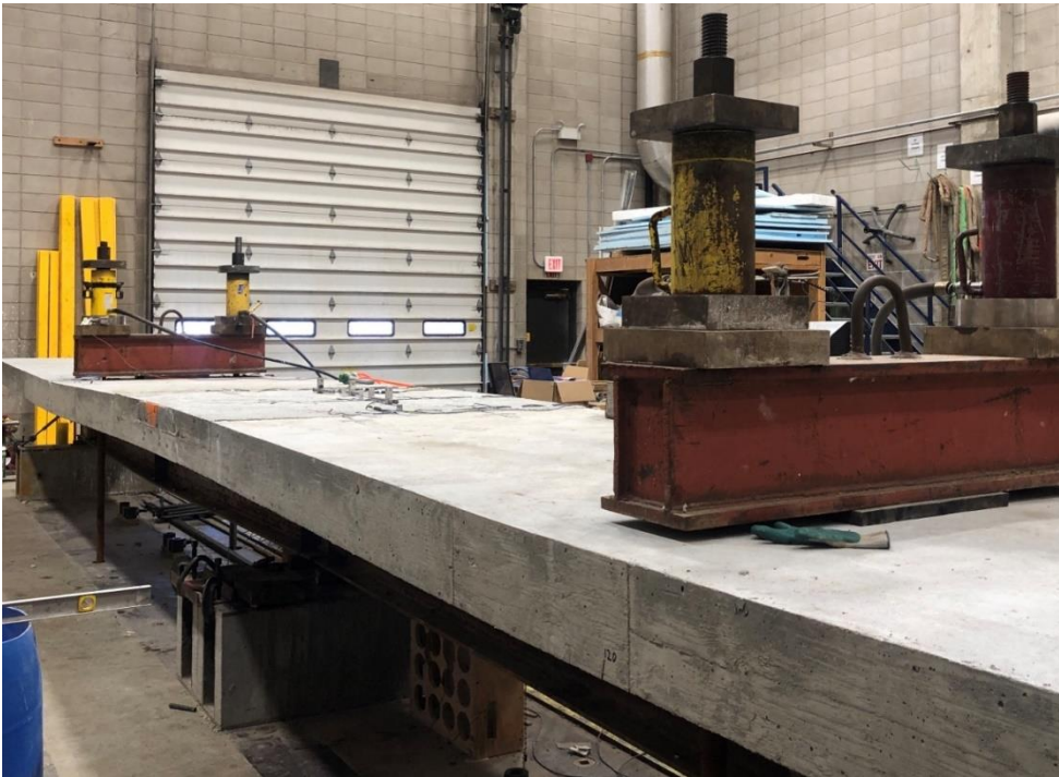
Figure 3.2 The Laboratory test setup, showing actuators at loading points.
