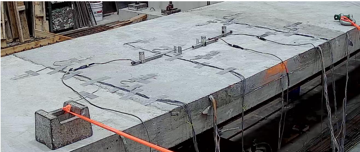
Figure 2.8 DCDT's and surface strain gauges on link slab 1
